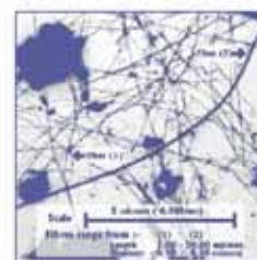
Straight Chrysotile Fibres in AC, magnification x 6500 (OEDA, 2002:2).
